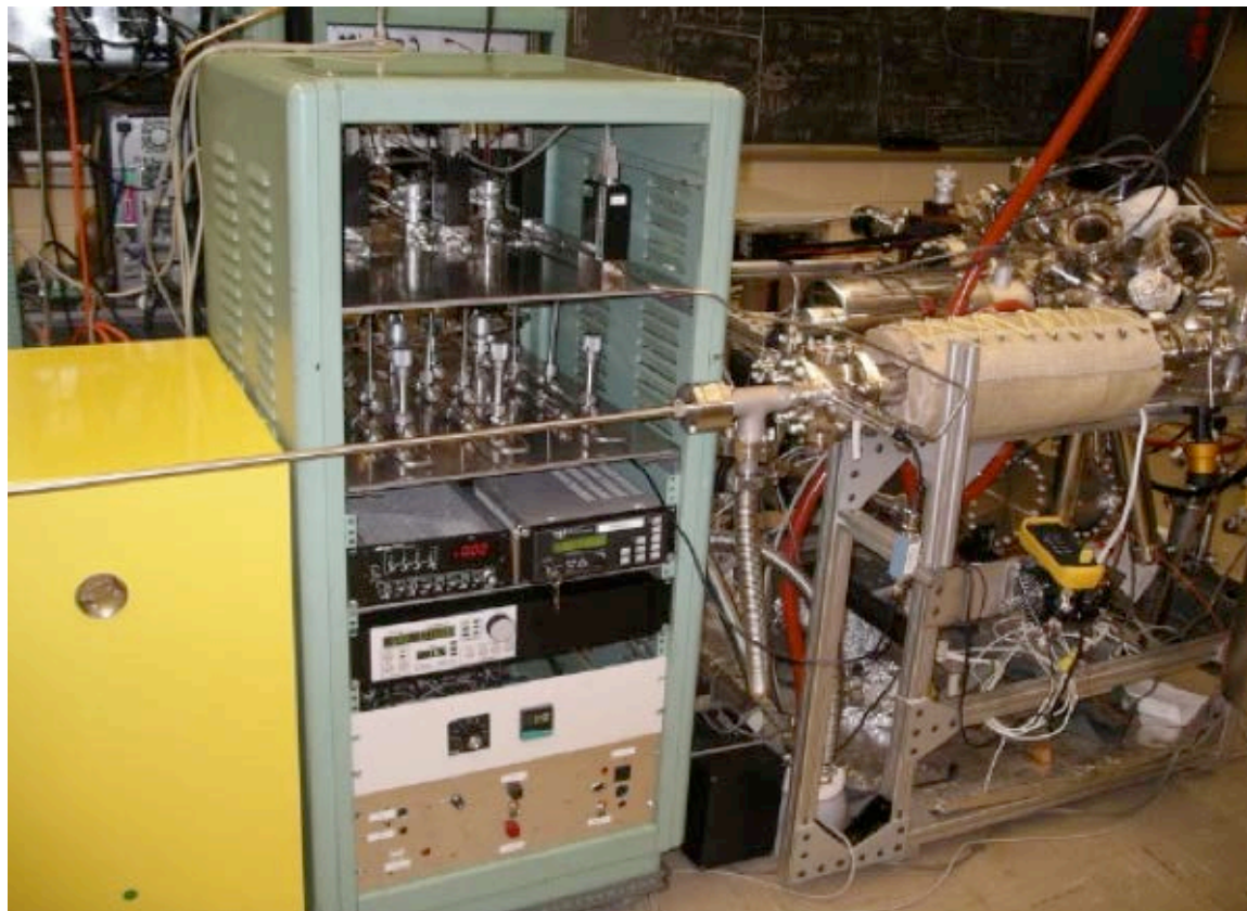
Figure 3.13 Viscous-flow UHV-interfaced ALD reactor with in-situ QCM.
